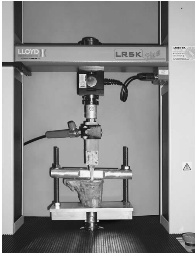
Figure 4. Tensile testing was performed in a uniaxial testing frame (LR5K-plus, Lloyd Instruments, Great Britain). The hamstring grafts were friction locked in a custom-made cryofixation clamp. All loads were applied parallel to the longitudinal axis of the bone tunnel to simulate a worst-case scenario.
