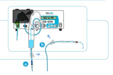
a: Connect the tube marked INFLOW to the arthroscopic scope sheath.
