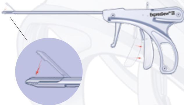
Close the jaw in preparation for use by pulling the jaw lever.
