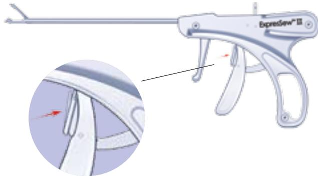
3. Open the jaw by pushing the jaw release button.
