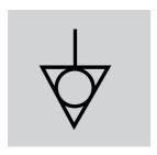
This symbol indicates the conductor that may be used to provide potential equalization between the equipment and the installations busbar.
