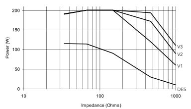
Note (1): Desiccate Full Power 120W Load/Ohms 3A Limit prevents 10R measurement
